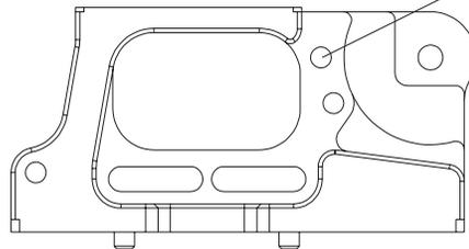
Use the top hole for loose tension
