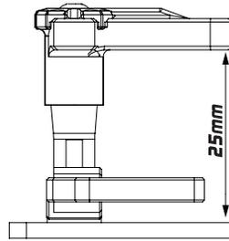
Freely Adjust Height Of Post With Shims,
